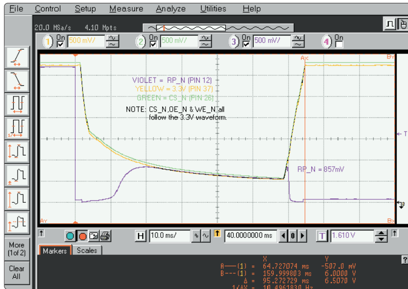
Figure 5. With a temporary capacitor added to prevent the 3.3 V from dropping into a range that sent the memory module into an indeterminate state, the module began generating valid data.
